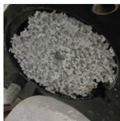
Unprotected and premature transom & outdrive zinc loss
