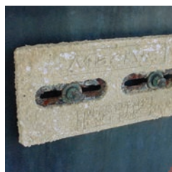
Unprotected and premature transom & outdrive zinc loss
