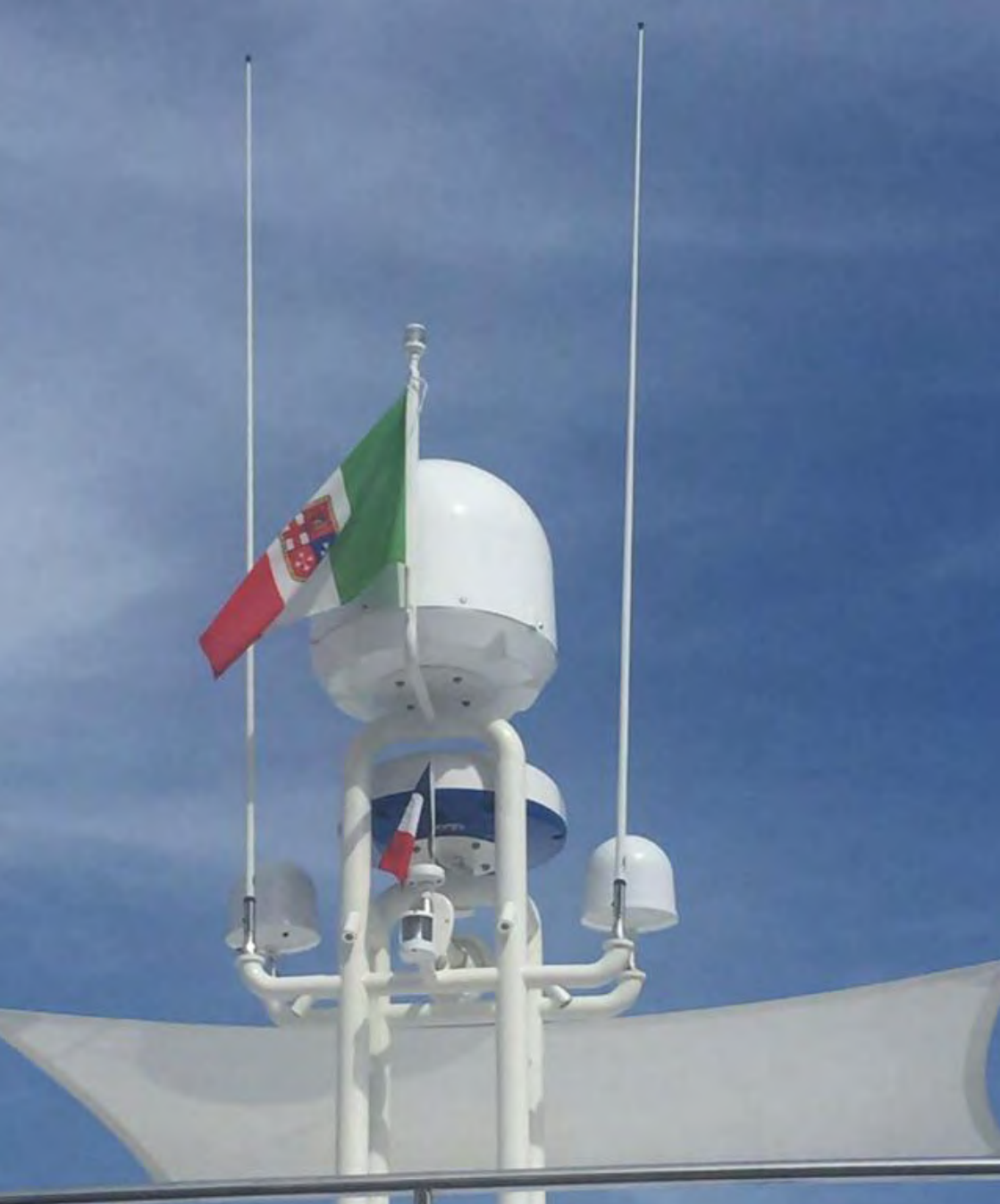
Glomex antennas - from left to right: 2.4m/8' High performing VHF antenna (model RA1225), weBBoat 4G Plus (the Dual Sim Coastal Internet antenna system), Rhea (47cm/18,5" DVB-S2 Satellite TV antenna), Altair (Full HD DVB-T2 TV antenna) and 2,4m/8' AM-FM radio antenna (model RA1288)
