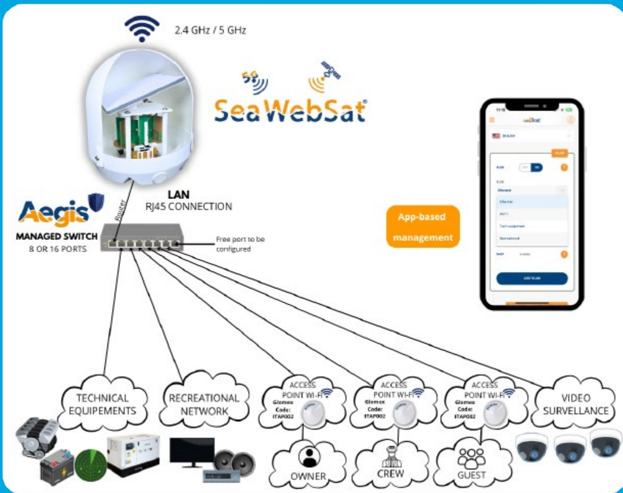
Onboard network setup example with SeaWebSat® OMNIX VLANs
