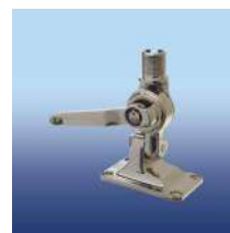
▲ RA116/SS 4 way ratched mount in stainless steel, handle locking, hole for cable, standard thread 1"x14
