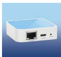
▲ ITAP001 Access point for metal/large boat.
