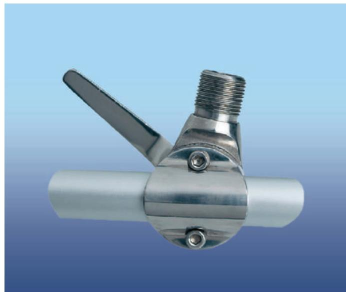
🇬🇧 Rail ratchet mount stainless steel electropolished, design with handle locking and hole for GPS. Easily installation on vertical or horizontal rails of 7/8" (22mm) and 1" (25mm). Usable with antennas no longer than 8' (2,4 m) in self supporting mode. Standard thread 1"x14 .
