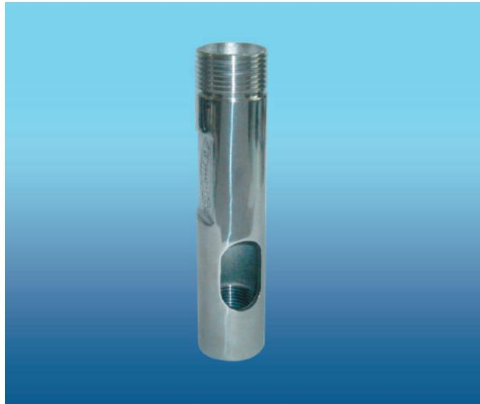
🇬🇧 Electropolished AISI316 stainless adaptor 1"BSP x 11 tpi male to 1"x14 UNS female - with slot for cable.
