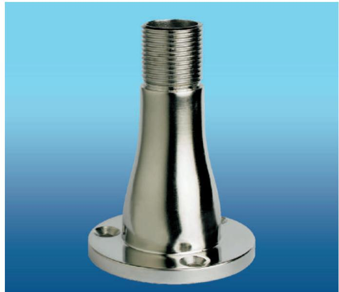
Universal mount stainless steel for antennas and extensions. Standard thread 1"x14, weight 10 oz (280 g), height 4" (100 mm).
