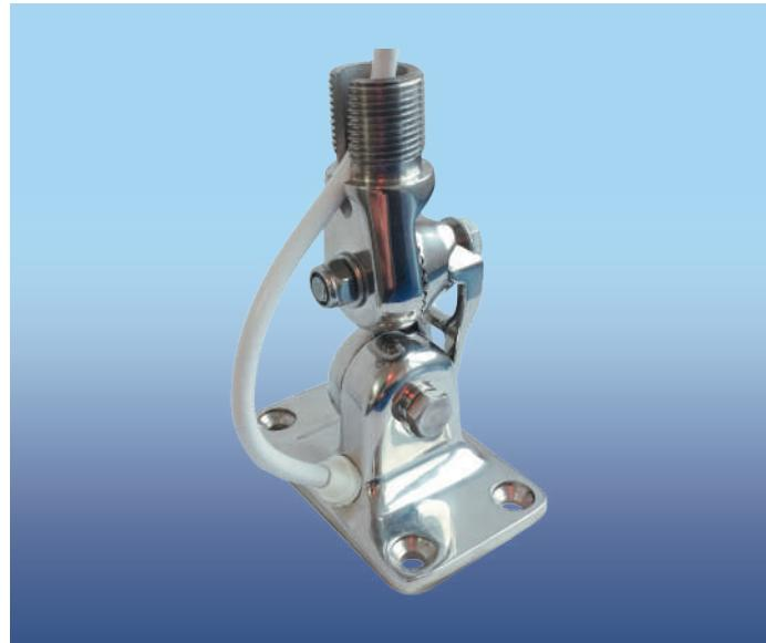
UK 4 way ratchet mount polished stainless steel design with clamp. Hole and feed-thru for coax cable. Standard 1"x14 thread. With special cable slot for a very easy passage of the cable without removal of most factory installed connectors
