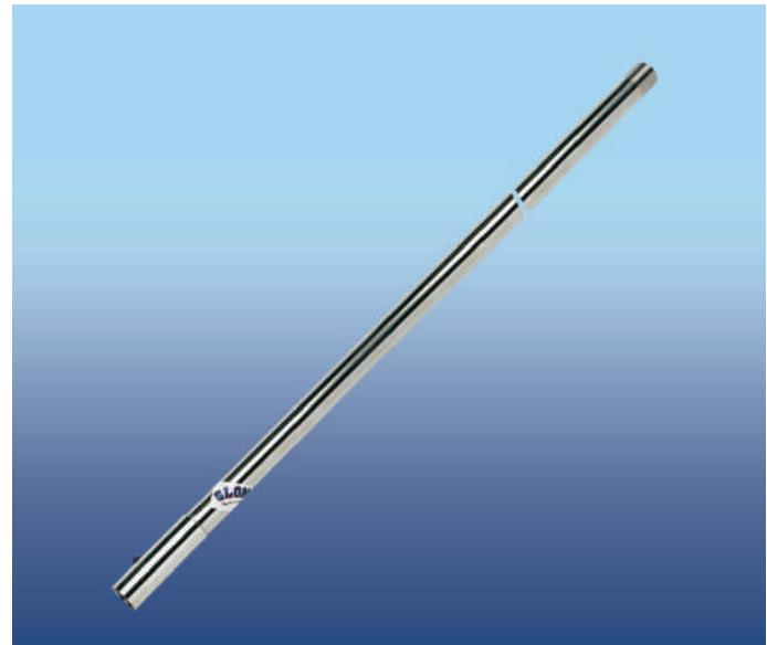
🇬🇧 Glomex antennas' extensions are used for vertical elevation of the antenna in order to clear the reception/transmission field. They can be made of stainless steel or UV resistant fibreglass, with standard 1"x14 thread on both sides, and they are the ideal complement to all Glomex antennas (VHF, AIS, etc.). NOT FOR GLOMEASY ANTENNAS RA123 is a stainless steel extension, 1,5 m/5' high.
