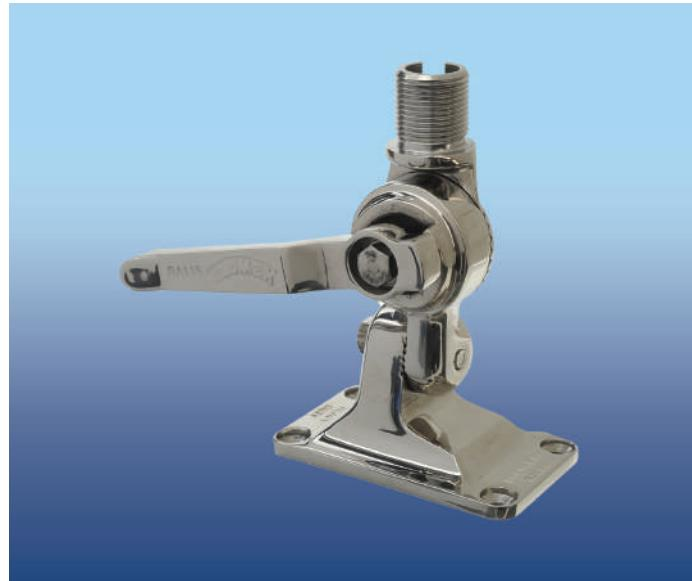
Heavy duty 4 way ratchet mount polished stainless steel design with handle, for deck or bulkhead. Hole for GPS and feed-thru for coax cable. Standard 1"x14 thread.
