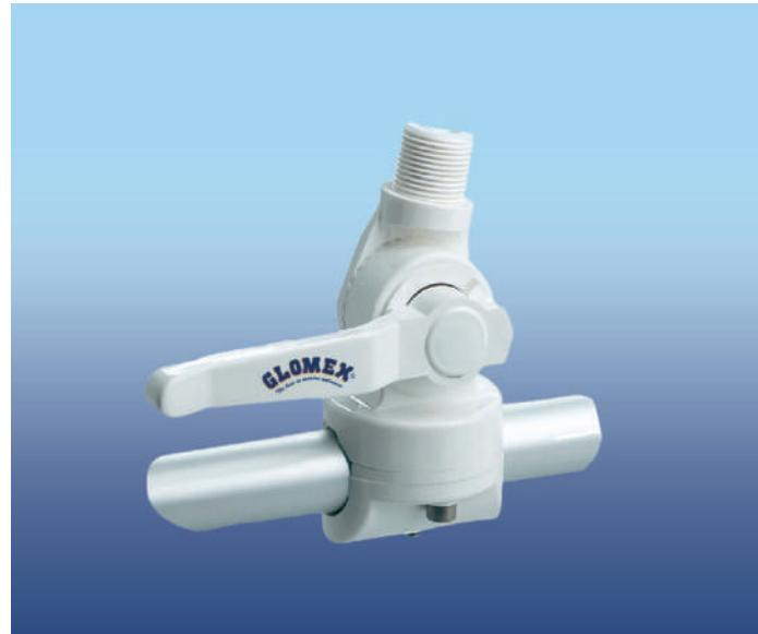
🇬🇧 Rail swivel mount in reinforced nylon UV resistant, design with handle locking and hole for GPS. Easily installation on vertical or horizontal rails of 7/8" (22 mm) and 1" (25 mm). Usable with antennas no longer than 8' (2,4 m) in self supporting mode. Standard 1"x14 thread.
