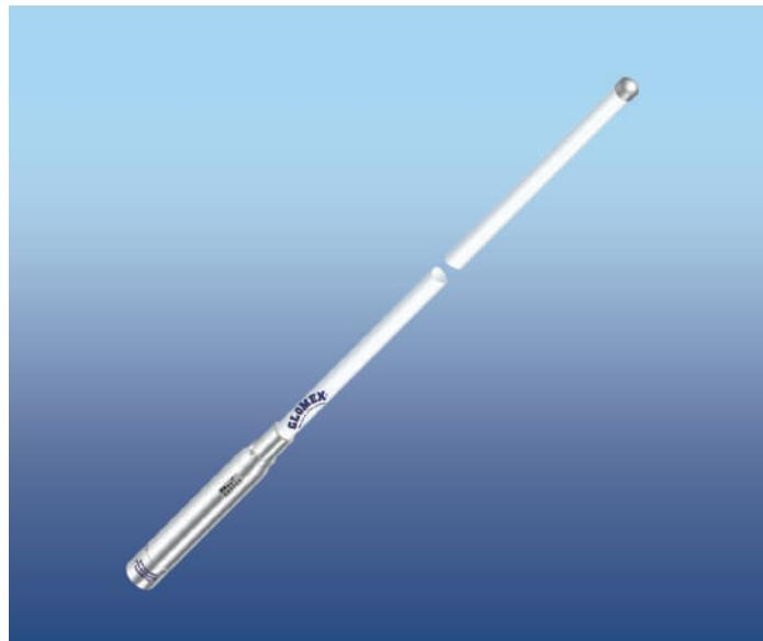
12 dBi gain antenna. Single Wi-Fi omnidirectional marine antenna (2.4 GHz). Integrated transmitter, powered by Bullet POE supplied. Easy mounting using 1"BSP mounts (not included). Termination: RJ45 10/100 base T Ethernet IEEE802,3. Vertically polarized, vibration proof, lightweight, corrosion resistant antenna.
