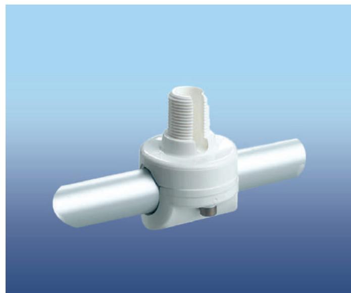
🇬🇧 Rail mount in reinforced nylon UV resistant, for installation of GPS antennas on horizontal rails of 7/8" (22 mm) and 1" (25 mm). Usable with RA129 extension. Standard 1"x14 thread.
