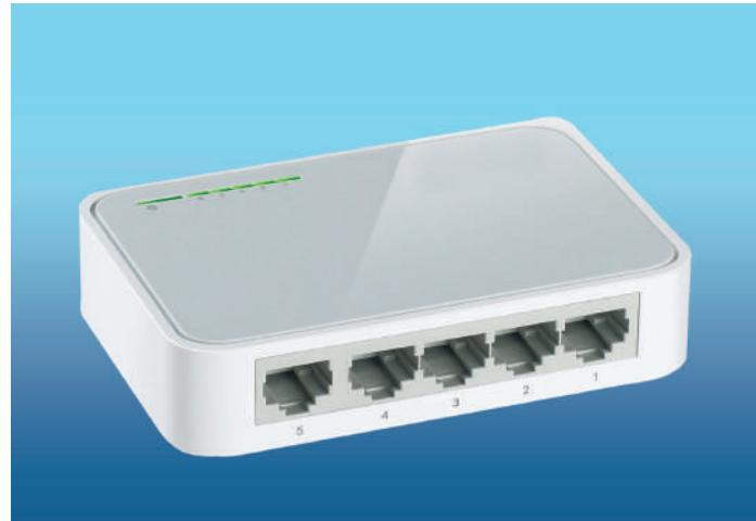
🇬🇧 5-Port 10/100Mbps Desktop Switch. It provides an easy way to expand your wired network. It can process data at a rate of up to 200Mbps making it an ideal choice for expanding your high performance wired network. Moreover, all ports support Auto MDI/MDIX Function, eliminating the need for crossover cables or Uplink ports
