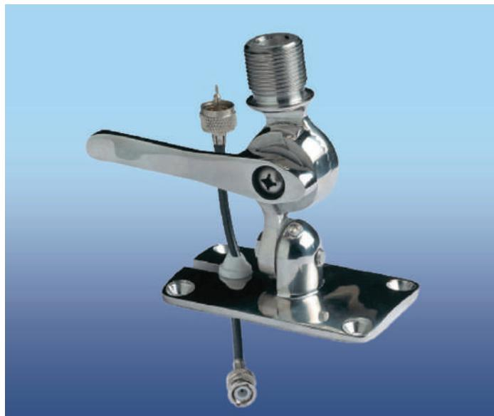
● 4 way ratchet mount polished stainless steel design with handle locking, for deck or bulkhead. Hole for GPS and feed-thru for coax cable. Usable with antennas no longer than 9' (2,7 m) in self supporting mode. Standard 1"x14 thread.
