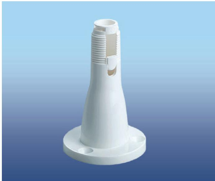
● Universal mount reinforced nylon for GPS antennas only. Usable with RA129 extensions. Standard thread 1"x14, weight 2 oz (50 g), height 4" (100 mm).
