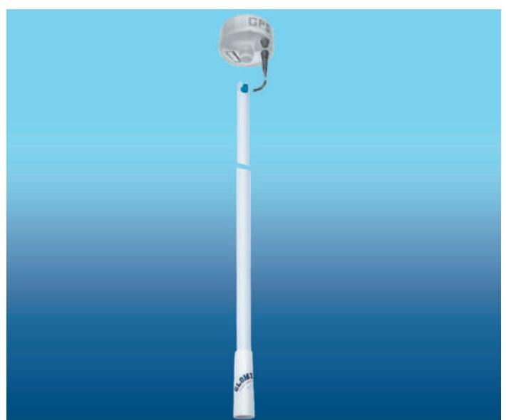
Alluminium extensions in glossy white paint for GPS antennas. They're available in various lengths, with standard 1"x14 thread, allow the central and side passage of the GPS antenna cable. RA129/120 is an extension 1,2 m/4' high.
