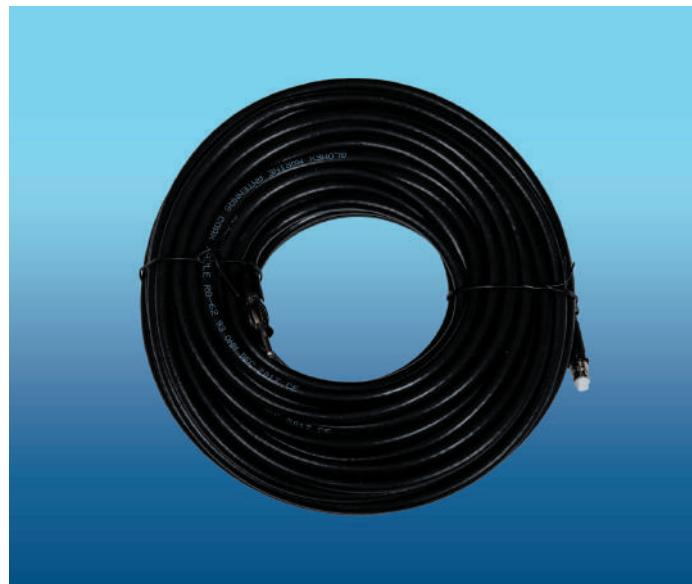
RG-62 low loss coaxial cable for Glomeeasy FM antennas. Long 6 m (20'), has pre-installed FME and Motorola connector for a very easy and fast intallation. This type of coaxial cable is available also in other lenghts: 18m (59') 25m (82').
