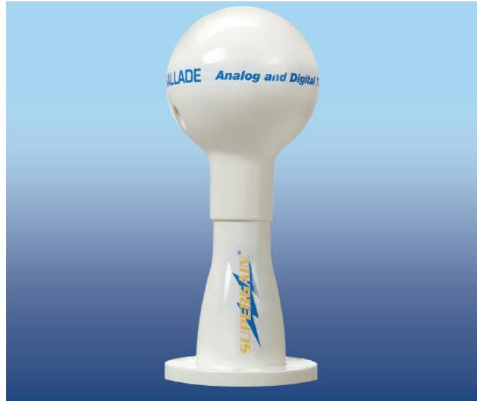
BALLADE is a 23,5 dB gain omnidirectional TV DVB-T2 / TNT and HDTV compatible antenna for boats and mobile vehicles: it's super-compact (70 mm / 2,8" diameter x 165mm / 6,5" height), extra light-weight (110g / 4oz) and easy to be installed thanks to the integrated mount.
