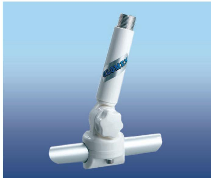
🇬🇧 Rail mount reinforced nylon UV resistant, design with knob locking, hole for GPS cable and extension 4" (100 mm). Easy installation on vertical or horizontal rails of 7/8" (22mm) and 1" (25mm). Usable with antennas no longer than 8' (2,4 m) in self-supporting mode. Standard thread 1"x14.
