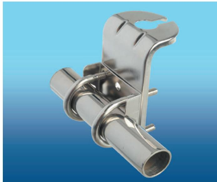
🌐 Antenna mounting bracket in stainless steel electropolished. For horizontal and vertical mounting on rail diameter 7/8" (22 mm) to 1 1/4" (30 mm). Standard thread 1"x14.
