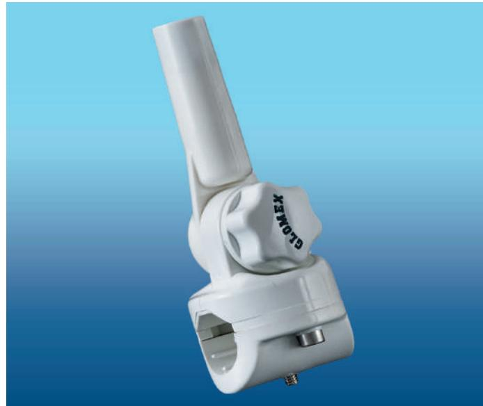
🇬🇧 Rail ratchet mount in reinforced anti-yellowing nylon UV resistant for Glomeeasy antennas, locking by knob Easy installation on vertical and horizontal rails of 7/8" (22 mm) and 1" (25mm). 5/8"x24 thread.
