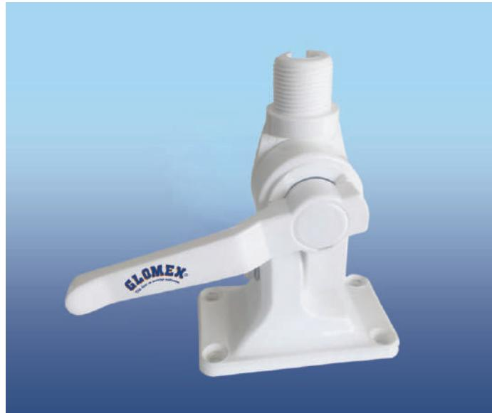
● 4 way ratchet mount in reinforced nylon UV resistant design with handle locking, for deck or bulkhead. Hole for GPS and feed-thru for coax cable. Usable with antennas no longer than 9' (2,7 m) in self supporting mode. Standard thread 1"x14.
