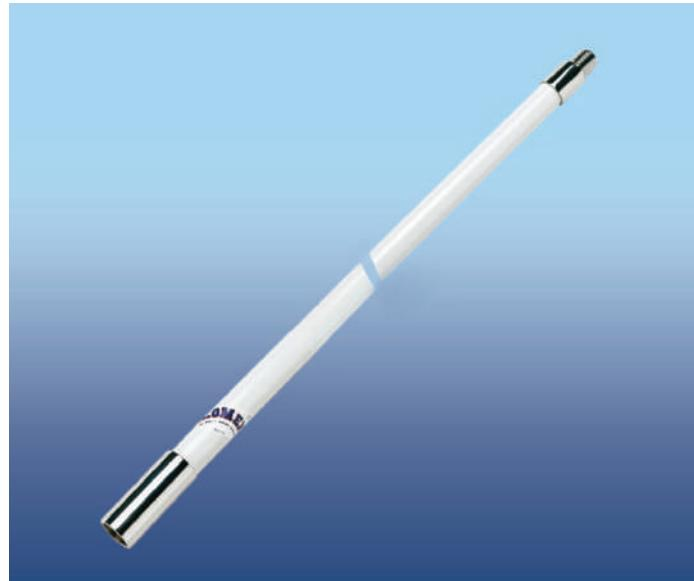
🇬🇧 Glomex antennas' extensions are used for vertical elevation of the antenna in order to clear the reception/transmission field. They can be made of stainless steel or UV resistant fibreglass, with standard 1"x14 thread on both sides and they are the ideal complement to all Glomex antennas (VHF, AIS, etc.). NOT FOR GLOMEASY ANTENNAS LINE RA149 is a fibreglass extension, 1.2 m/4' high.
