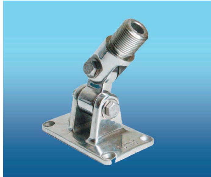
● 4 way stainless steel free swivel mount for any mounting location. Designed for a quick antenna lowering, it must be coupled with a stand-off bracket. Standard 1"x14 thread. RA176 must be coupled with RA819 stand-off bracket (not included) for installing the following antennas: PRA800, PRA900 and PRA903. Moreover, RA176 must be coupled with RA119 stand-off bracket (not included) for installing the following antennas: PRA702, PRA703 and PRA601.
