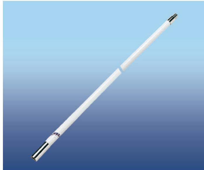
🇬🇧 Glomex antennas' extensions are used for vertical elevation of the antenna in order to clear the reception/transmission field. They can be made of stainless steel or UV resistant fibreglass, with standard 1"x14 thread on both sides and they are the ideal complement to all Glomex antennas (VHF, AIS, etc.). NOT FOR GLOMEASY ANTENNAS RA150 is a fibreglass extension, 2,4 m/8' high.
