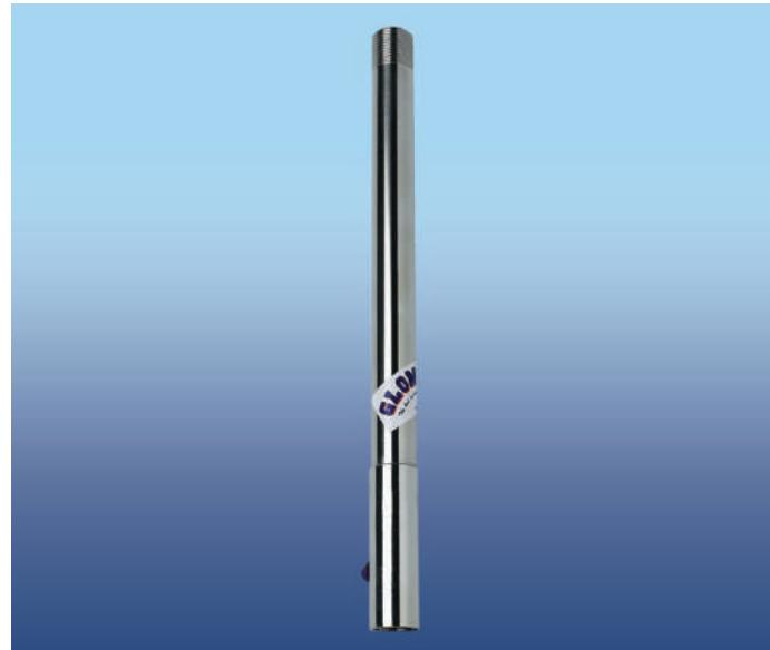
🇬🇧 Glomex antennas' extensions are used for vertical elevation of the antenna in order to clear the reception/transmission field. They can be made of stainless steel or UV resistant fibreglass, with standard 1"x14 thread on both sides, and they are the ideal complement to all Glomex antennas (VHF, AIS, etc.). NOT FOR GLOMEASY ANTENNAS RA103/30 is a stainless steel extension, 300 mm/12" high.
