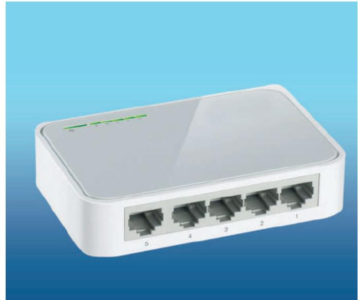
● 5-Port 10/100Mbps Desktop Switch. It provides an easy way to expand your wired network. It can process data at a rate of up to 200Mbps making it an ideal choice for expanding your high performance wired network. Moreover, all ports support Auto MDI/MDIX function, eliminating the need for crossover cables or Uplink ports.
