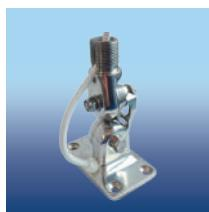
▲ RA107SSFME 4 Way ratcheted mount in stainless steel, locking by clamp, with cable slot, 1" x14 standard thread
