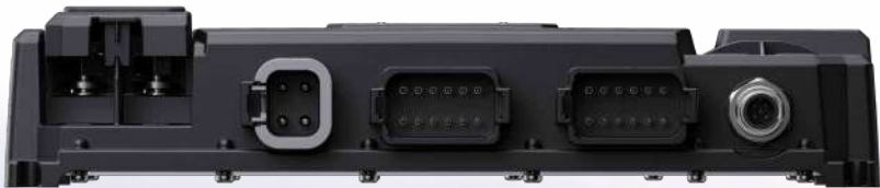
Bottom view showing moulded in Deutsch receptacles
